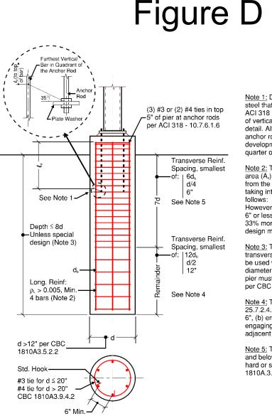
Note 1: Development length of vertical reinforcing steel that engages the anchor rod,  $\ell_a$ , must meet ACI 318 Section 25.4. It is measured from the top of vertical bar to the point shown in the enlarged detail. Alternatively, the embedment depth of the anchor rod may be determined as the development length of the vertical bar plus one quarter of the pier diameter ( $\ell_d$  + d/4).
